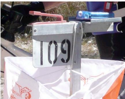
Inserting an SI-stick into the SI unit at a "stand" type control
