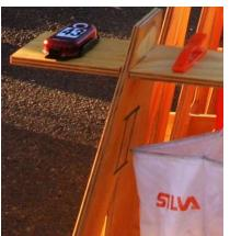
To record your time at each control, insert your Sportident stick into the hole; You will hear a "beep" and the control will flash red. If using a SIAC stick, wave it over the control and listen for the beep from the stick. The tip of the stick will flash red.
