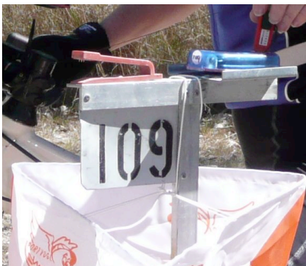
Inserting an SI-stick into the SI unit at a "stand" type control
