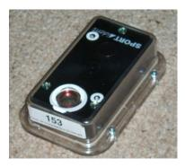
When the pCard is swiped or held over the hole in the control box and when the competitor hears a **BEEP** (also sees a flash) the pCard has recorded their time at the control.
